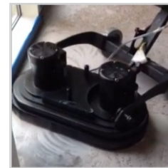
Offset Head Reaches Into Corners
